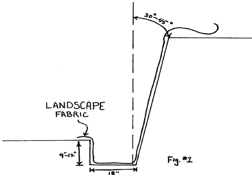
In dense or clay soils or in areas that do not drain well, excavate 10 to 12 inches deep and add 4 to 6 inch deep crushed aggregate. You should use an aggregate with good drainage quality as well as structural support. Directly behind the wall at the base install a drainage-perforated pipe wrapped with a drainage fabric with at least 3 inches of drainage rock all around it. (Fig. 2) Level the drainage bed with a rake and tamp the aggregate to compact it.
